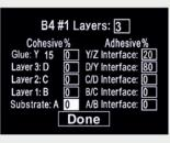
Record the pass/fail result and the nature of fracture - cohesive, adhesive, and glue failures - using the app (left) or the instrument's touch screen display (above)
